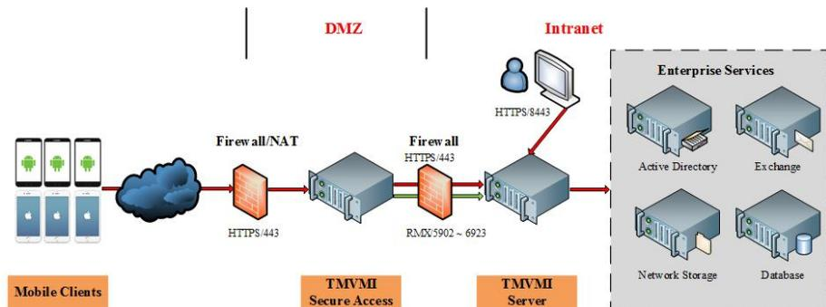
**FIGURE 1-1. Trend Micro Virtual Mobile Infrastructure Single Server Installation Model**
